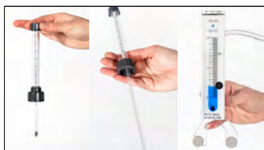
Thermometers gas & packing liquid, manometer (accessories)
