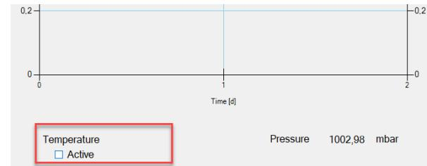
If the temperature measurement is active without a temperature probe being connected to the »SIM«, the measurement results of the gas volume will be incorrect.
