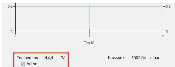
If a temperature measurement is not required or possible (**for example when the gas meter is placed in an ex-proof area**) the temperature measurement must be deactivated by clicking the tick box "Active":
